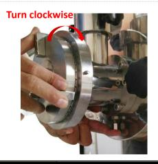
Push up the helical rod lock and hold it while turning the grinding disc clockwise to assemble it. Turn the grinding disc clockwise with the given wrench until feeling tight. Put on the front cap and tighten the securing knob.
