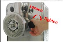
Loosen the hopper support securing knobs. Remove the hopper support.
