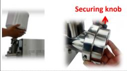
After removing the Hopper by loosen up the securing knobs, loosen the front cap securing knob to take off the front cap.
