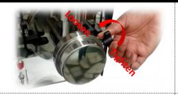
Loosen the front cap securing knob.
