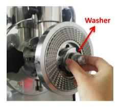
Choose the right washer and put it on the auger thread before installing the rotating disc. There are 4 washers to choose according to the fineness level required:
