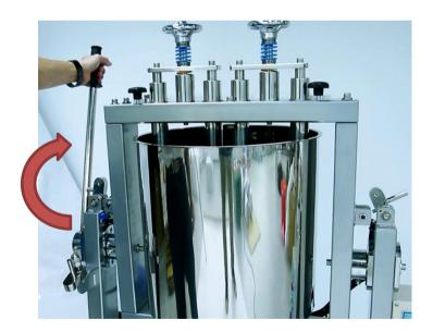
After discharging ingredient, open up the latch, and then push back the handlebar to tilt back the barrel to the upright position.
