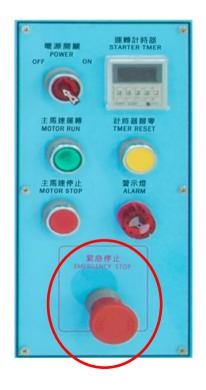
**Emergency Red Button** - located on the control panel (press it to stop immediately all actions)
