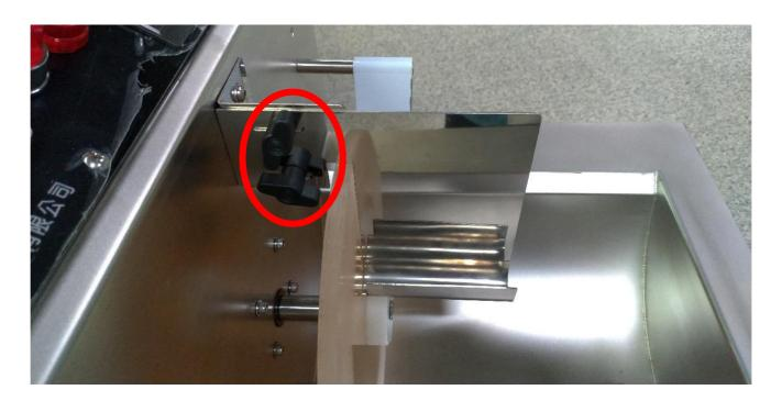
Step 2. Loosen up the nut of the rotating plate and remove the plate.
