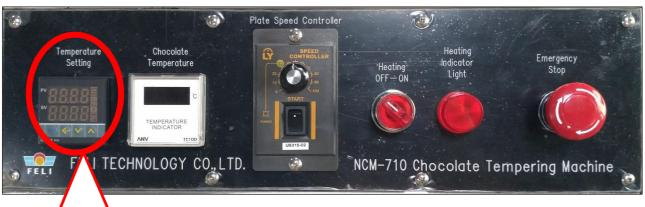
Adjust the water temperature setup
