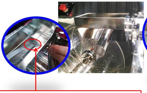
2. Adjust the height of the INJECTION DEVICE to keep it from touching the ROTATING PLATE so that it doesn't give impacts on the functioning of the ROTATING PLATE. Screw up the INJECTION DEVICE.
