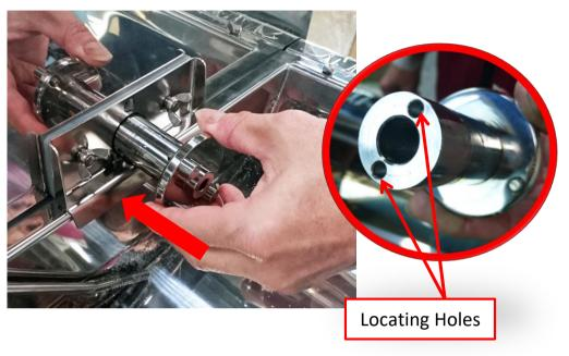
(Step 6) Reassemble the Rotating Plate
