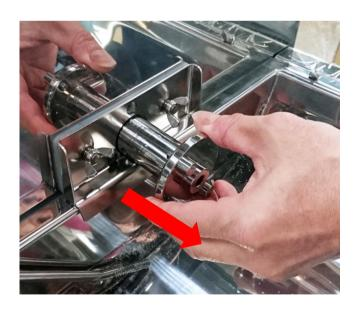
(Step 5) Reassemble the Axis for installing the Rotating Plate Insert the AXIS by aiming at the axial hole, and then turn around the AXIS in order for the locating holes on the end sides of the AXIS locate at the right position. The pins have to be inserted into the locating holes to complete the assembly of the AXIS, for installing the ROTATING PLATE later.
