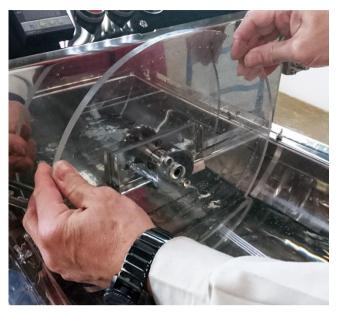
(Step 4) Disassemble the Axis Pull out the axis in a parallel direction.
