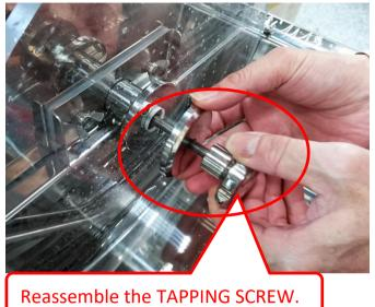
(Step 8) Reassemble the Injection Device Loosen up the TAPPING SCREWS circled on the photos and then lift up the INJECTION DEVICE to remove it.
