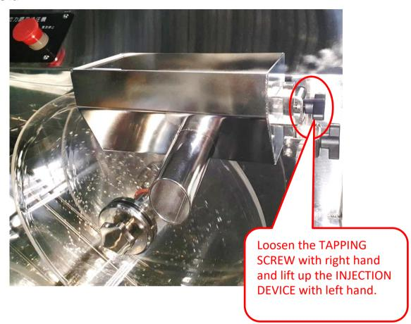
(Step 2) Disassemble the Screws for the Rotating Plate Loosen up and remove the TAPPING SCREW for the ROTATING PLATE circled on the photo.
