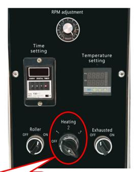
Set up the numbers of the heating tubes.
