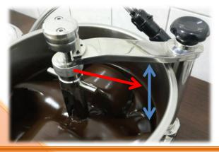
Press downward the rod to turn off the heater.
