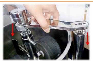
4. Install the positioning support. (Align one end with the positioning hole and align the other end with the two positioning rods. Put pressure on the positioning support and verify if the positioning support is well installed.)
