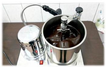
3. Turn on the machine to start the refining process. It is not a requirement but an option to put on or not the transparent lid.
