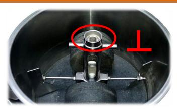
2. Place the granite wheel support inside the pot vertically with the positioning hole facing upward.
