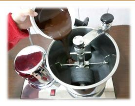
2. Add cocoa paste into the pot. Do not let the cocoa paste exceeds the height of the stone mill.
