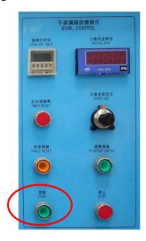
Step 4: Set up the turning speed in RPM/ the monitor indicates the turning speed in RPM. The setting range is from 0 to 120.
