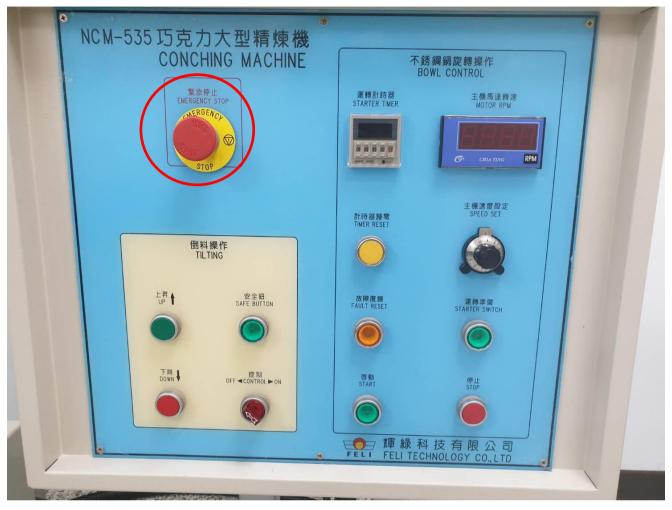
**Emergency Red Button** - located on the control panel (press it to stop immediately all actions)
